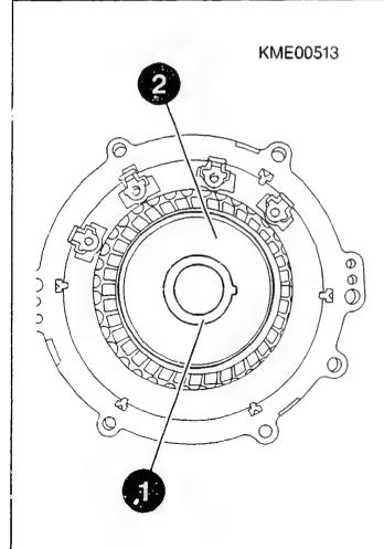
CHECKING AND REPAIRING ALTERNATOR Replacing NDE bearing (dismantling) Carefully clamp windingless rotor (1) in vice between soft jaws. ATTENTION: Clamp at shaft only. Use extractor to pull deep-groove ball bearing (2) off windingless rotor.
